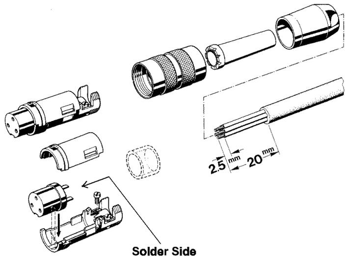
Figure 3. Female Cable Connector Assembly
