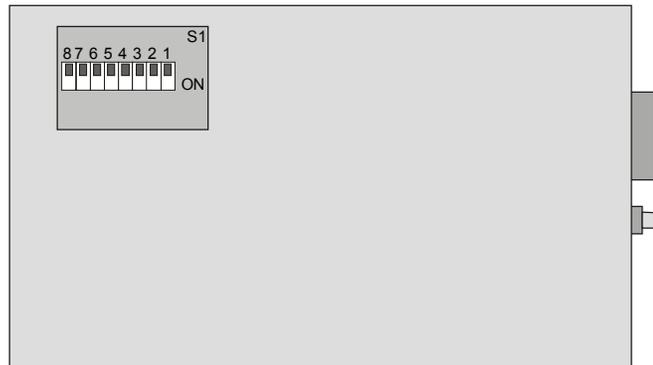
Figure B-3. DIP Switch Location
