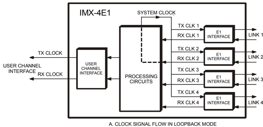
A. CLOCK SIGNAL FLOW IN LOOPBACK MODE
