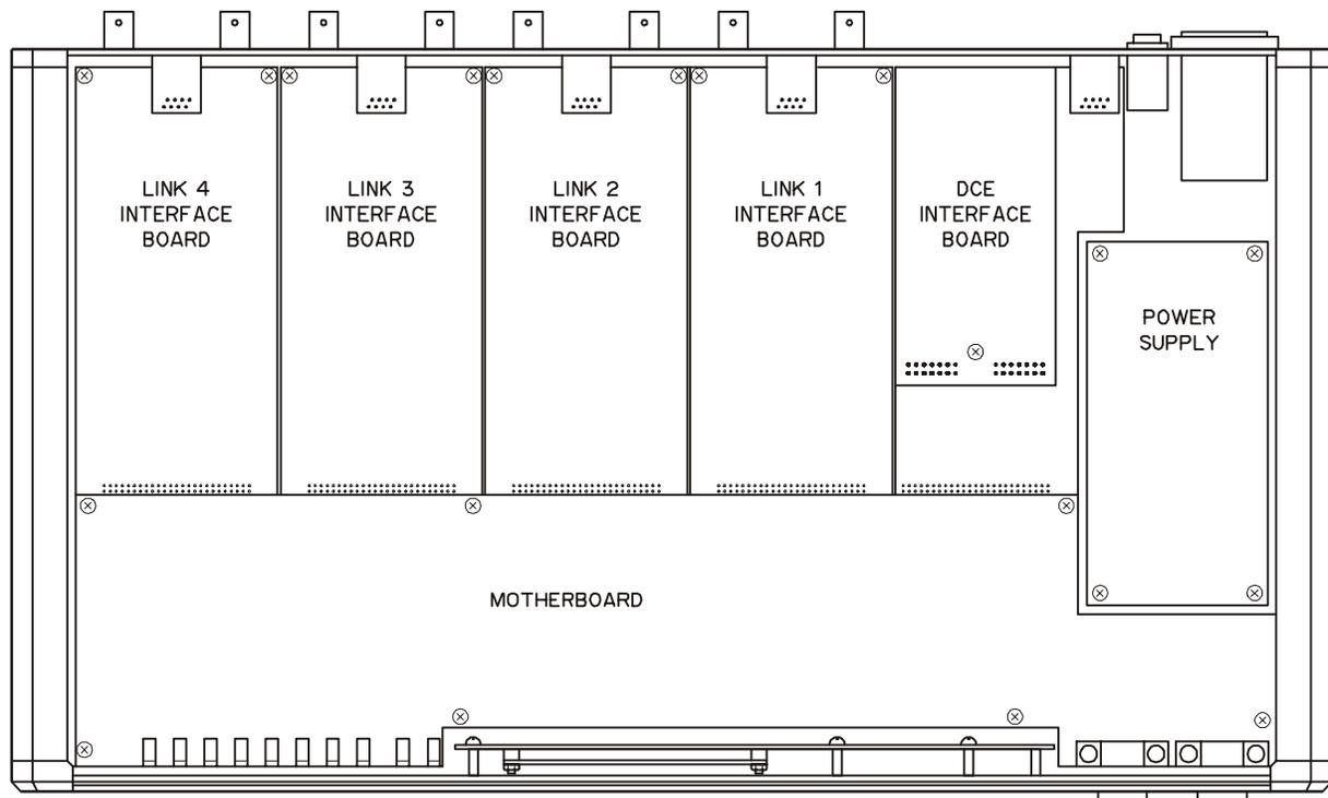
Figure 2-1. IMX-4E1 Construction
