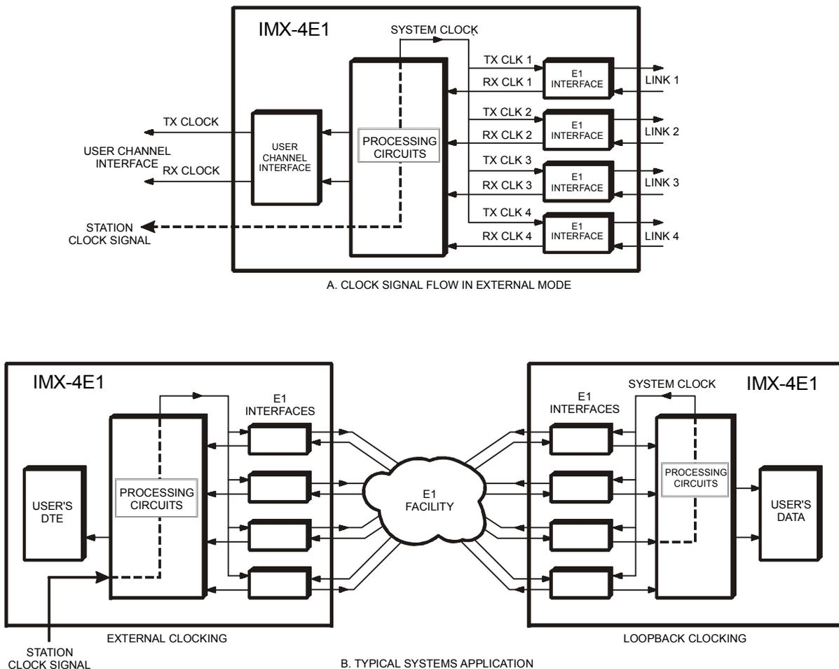
Figure 1-7. Flow of Timing Signals in External (Station) Timing Mode
