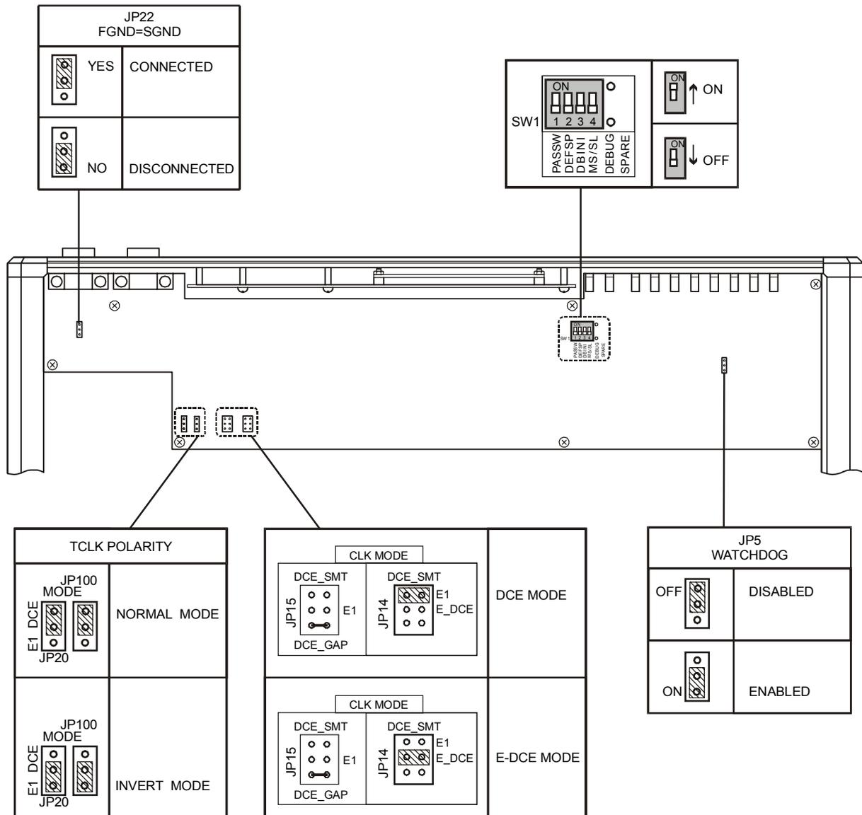
Figure 2-2. IMX-4E1 Motherboard, Internal Settings
