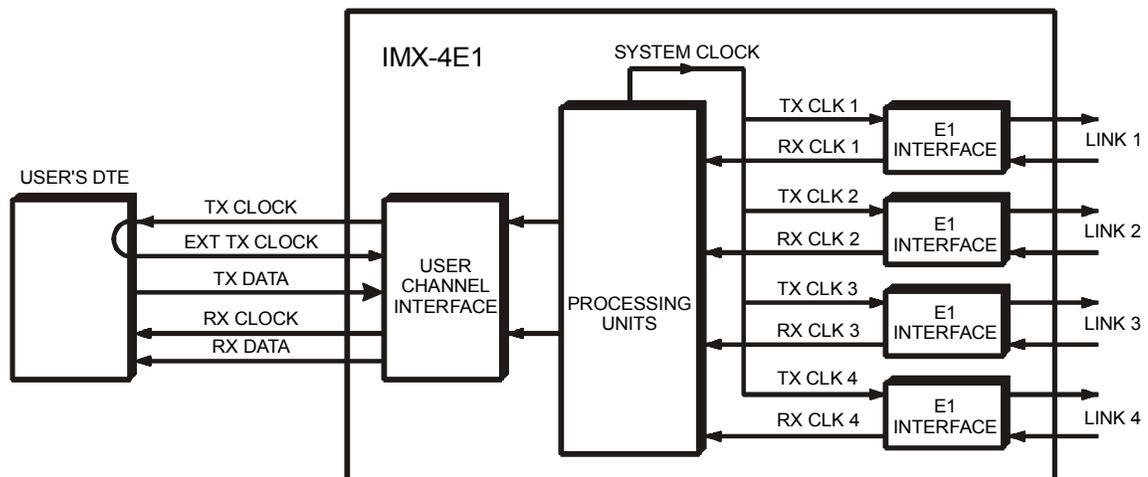
Figure 1-4. Flow of Timing Signals in User's Data Channel Interface in the E-DCE Mode
