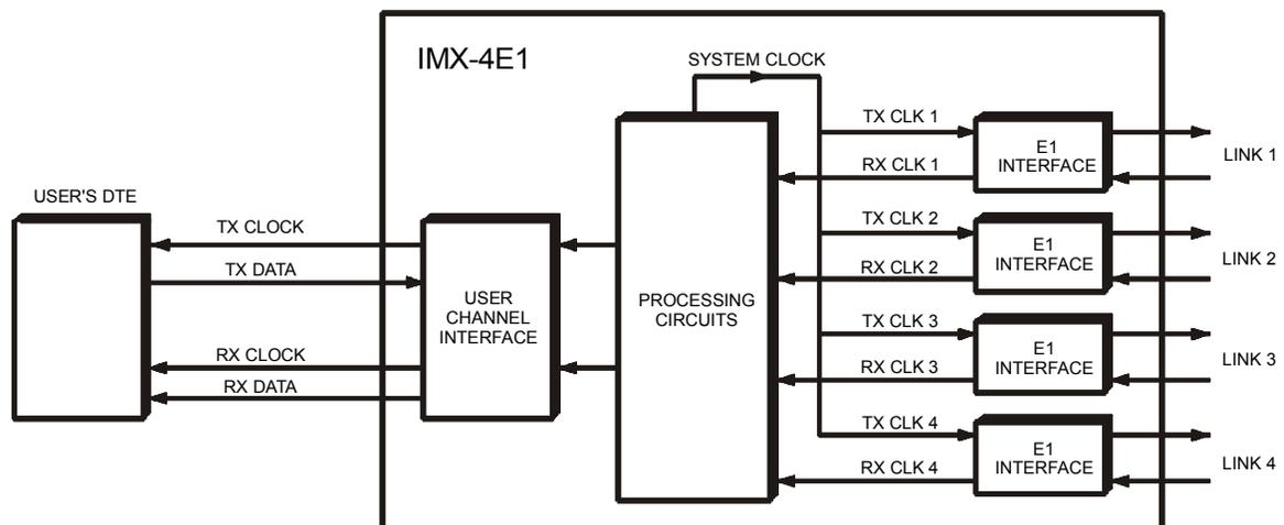
Figure 1-3. Flow of Timing Signals in User's Data Channel Interface in the DCE Mode
