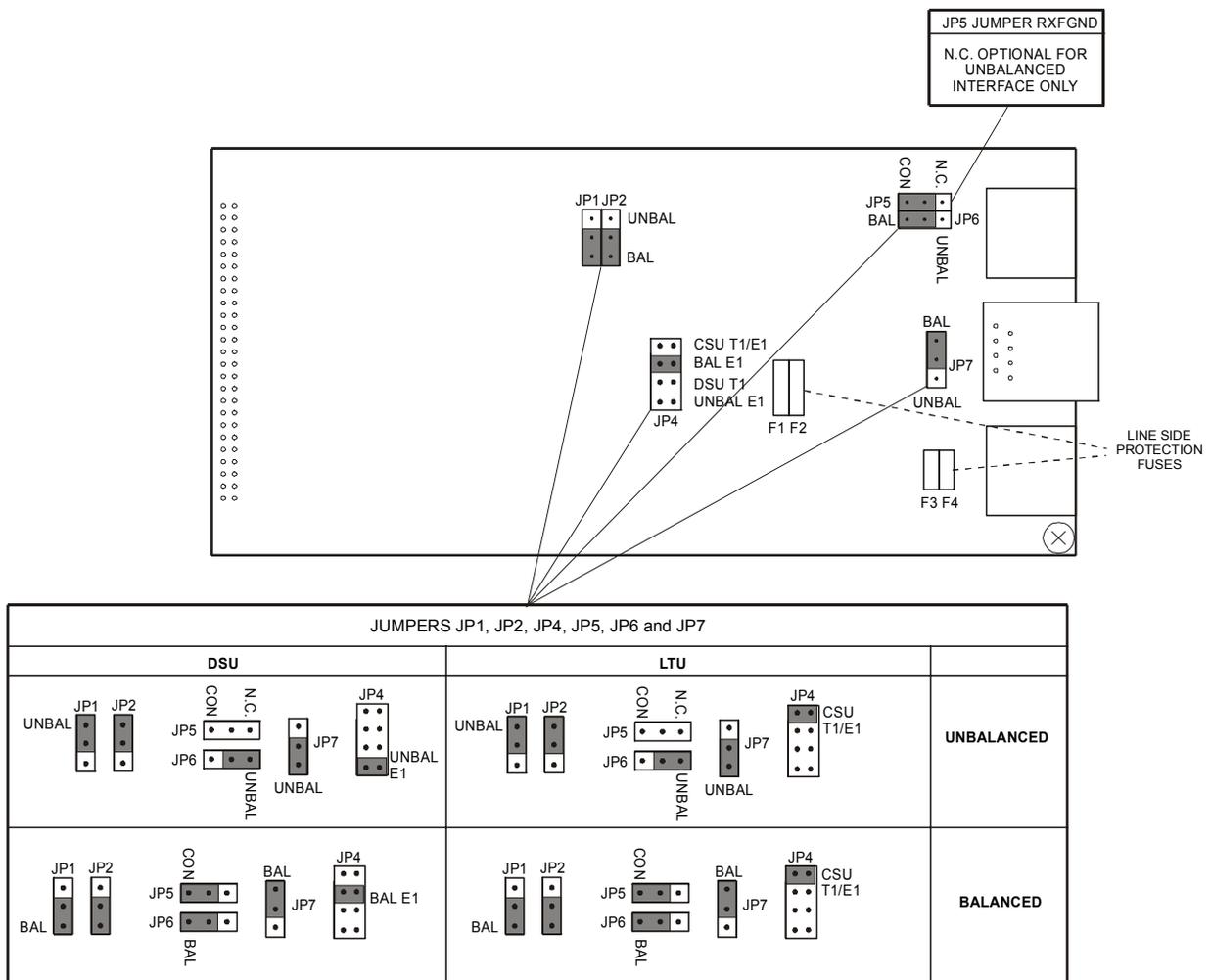
Figure 2-3. E1 Link Interface Board, Internal Settings
