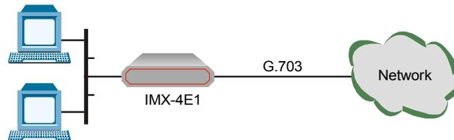
Figure B-1. Typical Application of IMX-4E1 with IR-ETH/QH Module
