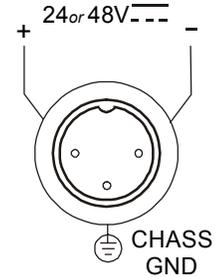
Figure 1. DC Power Input Connector (on unit panel)
